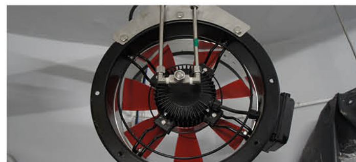
Dosing the formulation into the contaminated space utilizing a fan.
